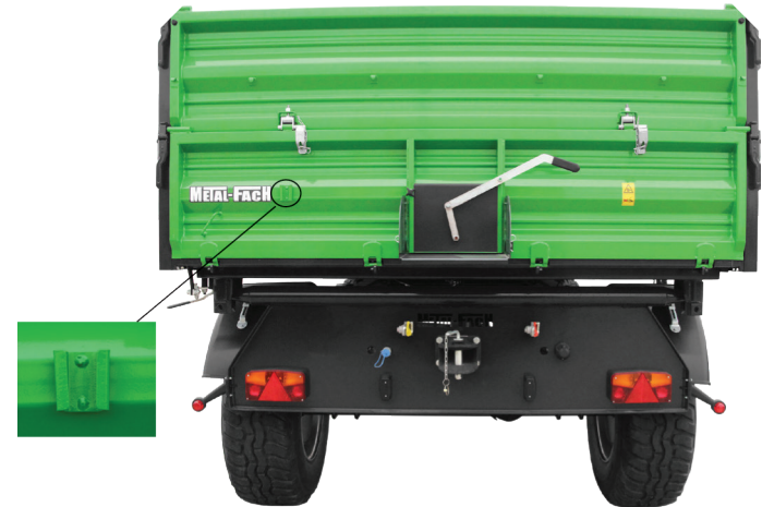
Fig. 4 Location of the bracket for the slow-moving vehicle sign.
